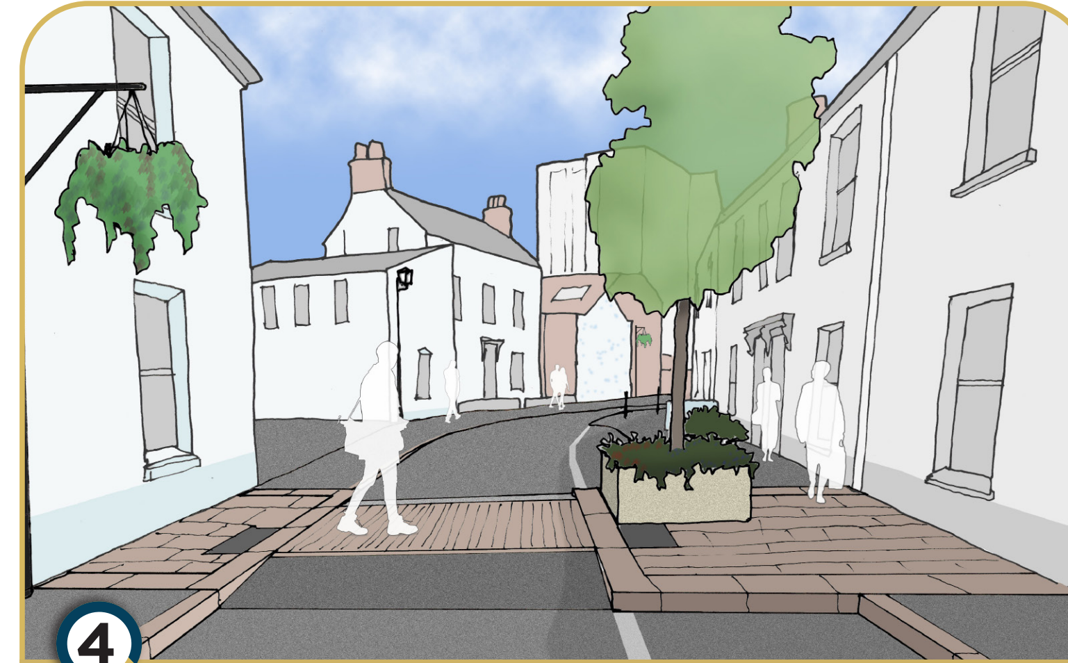
View looking south towards Dorset Street junction, showing resurfaced ramp and pedestrian crossing.
